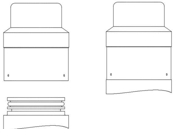
3. Push one dowel pin in each of the three holes in the housing. When the pins are fully inserted, the housing is permanently attached to the base.
