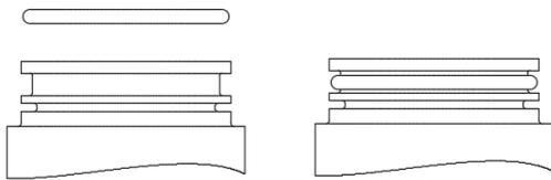
2. Slide the housing onto the base. Make sure that the o-ring does not get pinched, and that the housing is fully seated on the base.
